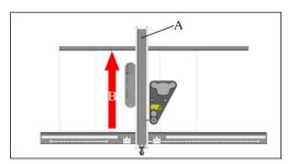
5. After placing the base in a suitable spot, rotate the locking handle until the locking screw is completely retracted. Check by hand that the base is securely attached.
