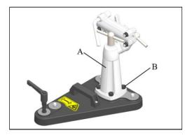
7. Insert feeder arm (A) in the arm holder (B).
