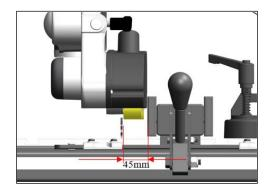
It is recommended using material 40 mm wide at maximum to avoid excessive resistance that may cause the base to shift and be unstable. Excessive resistance can be avoided by reducing saw blade speed or feed rate as well.
