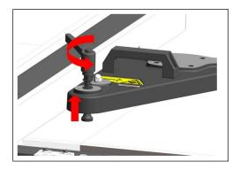
6. Use four screws M10 and four spring washers (B) to mount the feeder base (A) to the magnetic base. Use all four screws and washers to mount the base.
