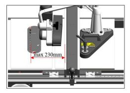
Minimum material width after cutting is 45 mm, otherwise the roller may be damaged.
