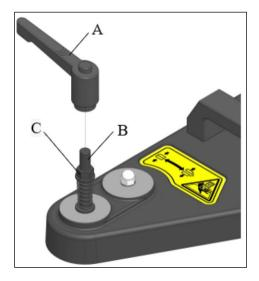
2. Rotate the locking handle (A) to protrude the locking screw (B). Now move the base to a suitable spot.
