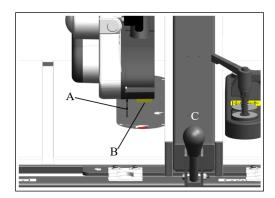
2. The feed roller should extend beyond the saw blade edge at the feed entry (C). The material must first touch the roller (B), then the blade (A).
