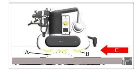
3. To feed the material correctly, the distance between the infeed roller (B) and fence should be 3 - 5 mm greater than the distance between outfeed roller (A) and fence.
