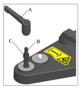
3. Disconnect the machine from the power supply! Remove blade guard (A) from the table saw and lower the saw blade (B) into the table.
