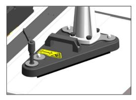
8. To move the base with mounted feeder, rotate the locking handle and lift the base from table surface.
