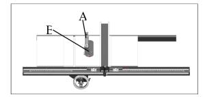
4. Adjust the rip fence (A) according to material size and place the magnetic base to the right of the feed direction (B). Before placing the base, check that the locking screw is extended.
